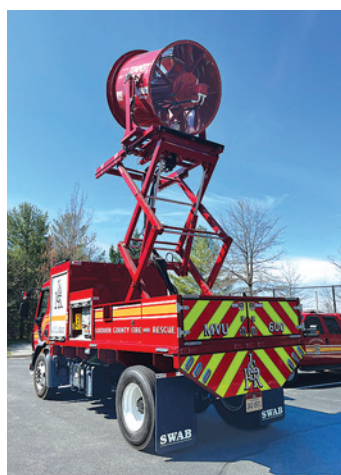
Loudoun County Fire and Rescue's MVU 600, a mobile ventilation unit that provides massive air movement, was used to remove carbon monoxide from Lovettsville Elementary School on February 9.
